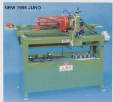
Juno 36", Will every make and type of professional cutting cylinder and bedknife. Can 'in-situ' grind many greensmower reels. Water cooled (eliminates dust and and fast to use, accurate 'relief angle' grinder
