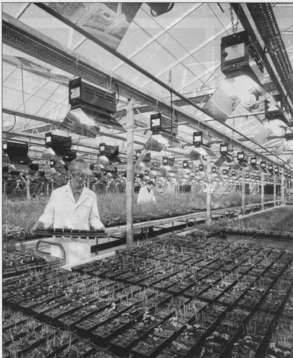
Potential active ingredients are tested in a 750m totally computer controlled glasshouse. The temperature inside is 22°C and the air is changed six times per hour
