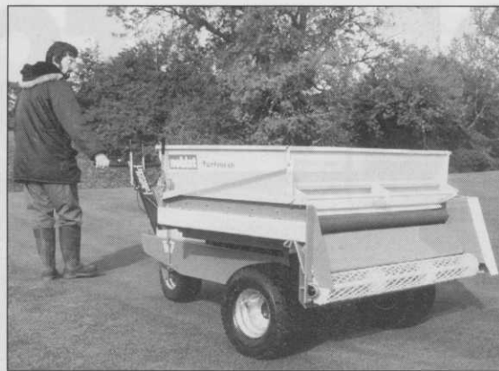
Turfmech Machinery's SAB 125A uses a patented rotating cage distributor at the rear to ensure even application without lumps
