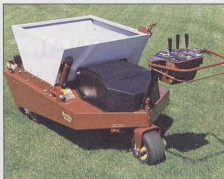
Above: Turfco Mete-R-Matic self propelled top dresser from Turf Machinery Ltd has a patented chevron belt conveyor for precise application of dry and damp materials at varying rates. Top: Able to carry up to 500kg of material, the Ultra Plant UP30 top dresser has a serrated roller and brush feed mechanism.
