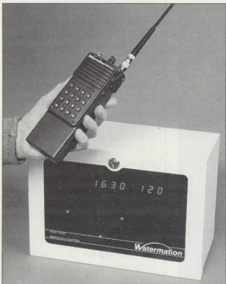
A Watermation TW2 4-zone controller with remote radio activation Picture courtesy of Watermation
