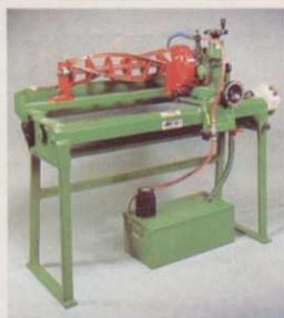
The new Juno 36" capacity Cylinder and Bottom Blade Grinder will accommodate every make and type of professional and domestic cutting cylinders and soleplates. Simple to operate, fast changeover from cylinder to bottom blade grinding.
