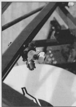
The triplet snap-fit interchangeable nozzle body fitted with diaphragm valves
