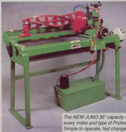
The NEW JUNO 36" capacity Cylinder and Bottom Blade Grinder will accommodate every make and type of Professional and Domestic cutting cylinders and soleplates. Simple to operate, fast changeover from cylinder to bottom blade grinding.
