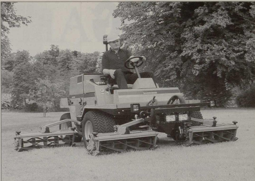
21 → world. The mower has no gearbox. Its transaxle is direct driven from the engine via a two-section hydraulic pump. One section drives the reel motors, the other supplies the steering and cutting units' lift rams. Apart from the 'Diesel' logo, the only visible difference between the petrol and diesel-engined machines is the rear hood which has been raised slightly to accommodate the taller power unit. Available next Spring, the JD 2243 diesel greens mower costs from £12,887.
