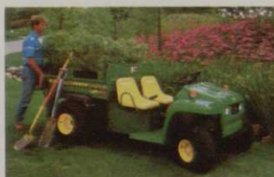
Both Gators feature high flotation, low pressure tyres for work on turf.
