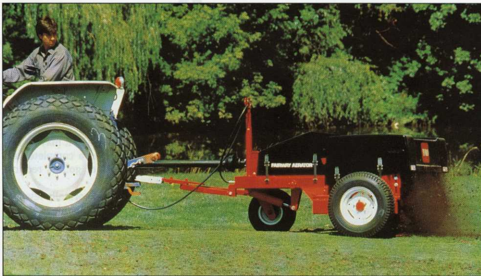
Above: Two hollow coring patterns can be selected on Toro's Fairway Aerator to deal with most turf aeration, thatch control and drainage needs across large turf areas. With a working width of 63in (1.6m) and workrate of 1.5 acres/hour, the machine can be set to work a maximum of 5in (127mm) deep behind tractors of 35 to 45hp.
