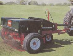
FAIRWAY AERATOR Now you can aerate fairways and other large turf areas up to 4 times faster than other reciprocating aerators. Our fairway aerator features a 160 cm (63") coring swath with multiple depths and coring patterns. It is capable of aerating up to 5,667 sq metres (61,000 sq ft) per hour and is designed for most 35-45 hp universal tractors. A coring head lock up stands secure head while transporting or servicing, and can be lifted and lowered hydraulically from the tractor seat.
