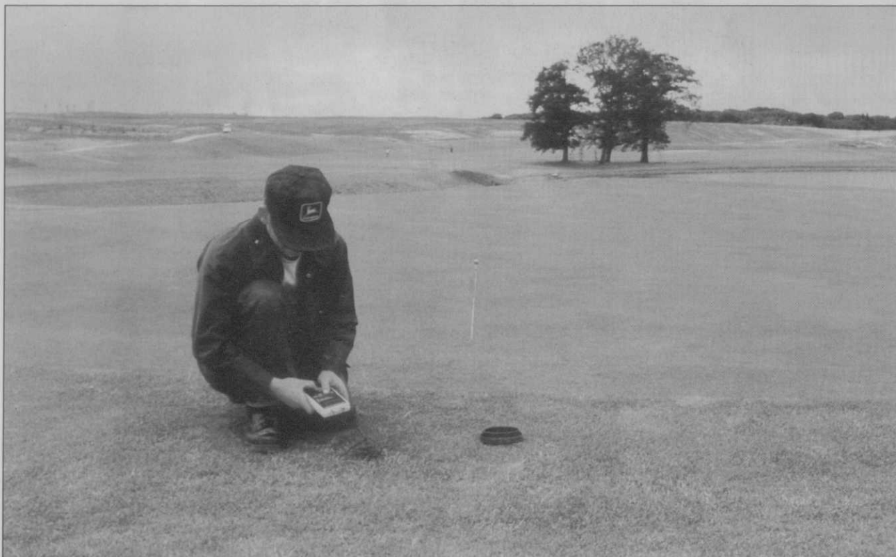
Taking readings, two or three times a week, with a meter, plus thermometer placed at 6" depth in the green
