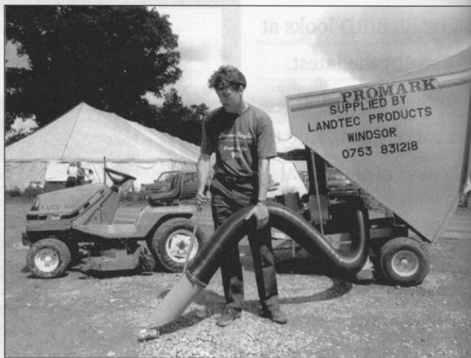
An engine-driven fan on Promark's 1050 Vacuum provides suction at a 1.5m pick-up head or through a 3m wander hose
