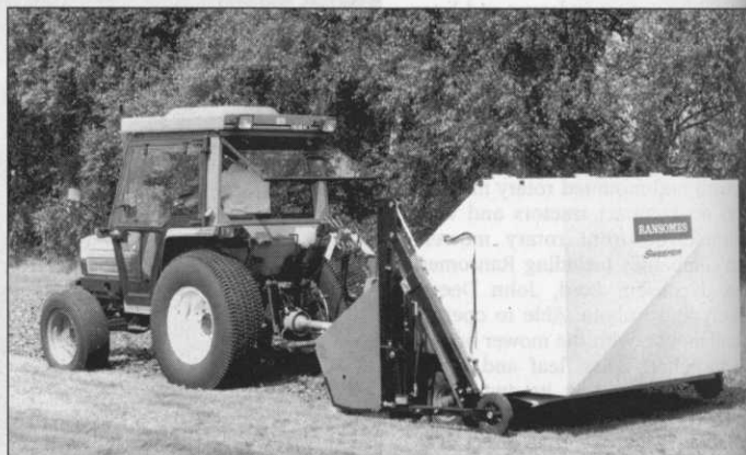
Ground clearance and brush pressure are controlled hydraulically on the Ransomes 2000 trailed sweeper. A scarifying reel is optional
