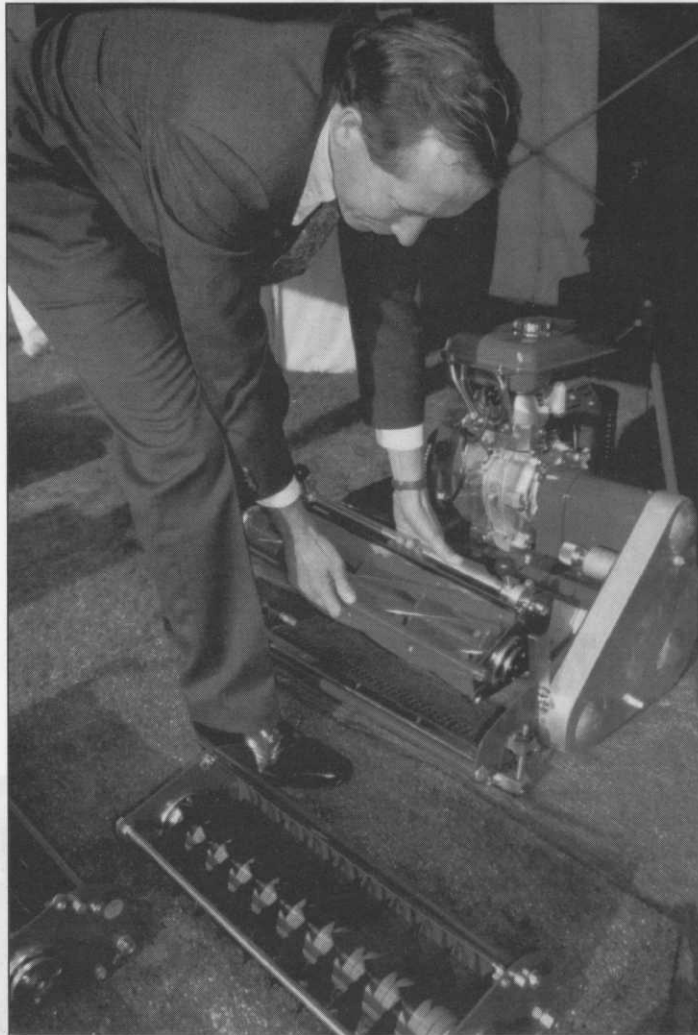
Ian Howard, Dennis's sales director, demonstrates the ease of removal of the interchangeable cassette head on the new FT510 mower
