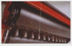
The HydroJect will aerate any soil type with high velocity water jets no matter how compacted. penetration to depths of between of their own 4" to 20" ... with virtually no turf surface distrubance
