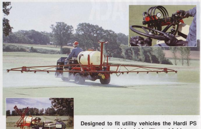
Designed to fit utility vehicles the Hardi PS sprayer has a 'drive in' facility and fold-away storage legs
