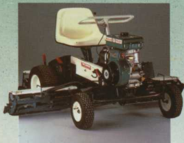
NATIONAL & 1990 Winner in GMA Annual Machinery Awards. Full 68" cut, folding side cylinders. 7 1/2hp Kawasaki engine.
