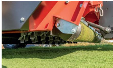
Above: The Redexim Turf Tidy with fully floating head.
