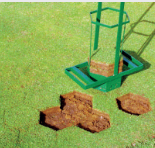
Figure 3 – Shows a hexagon turf doctor, this cuts the damaged turf areas and collects them in a stack. The damaged turf is disposed of and a similar number of new turves are cut from elsewhere (turf nursery) and these are slotted back into holes to replace the damaged turf. Image courtesy of Better Methods Europe Ltd www.BMSgolf.com
