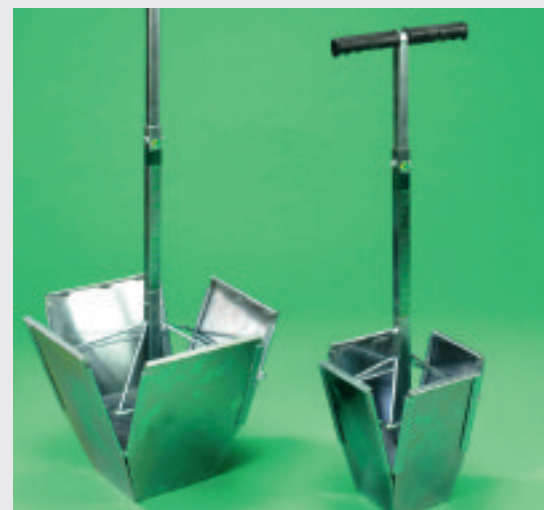
Figure 1 – Shows two different sized turf doctors. Note: The depth of core. This deep core means repairs are firm enough for players to walk/run over without the repairs coming loose. The deep roots mean the area soon establishes.
