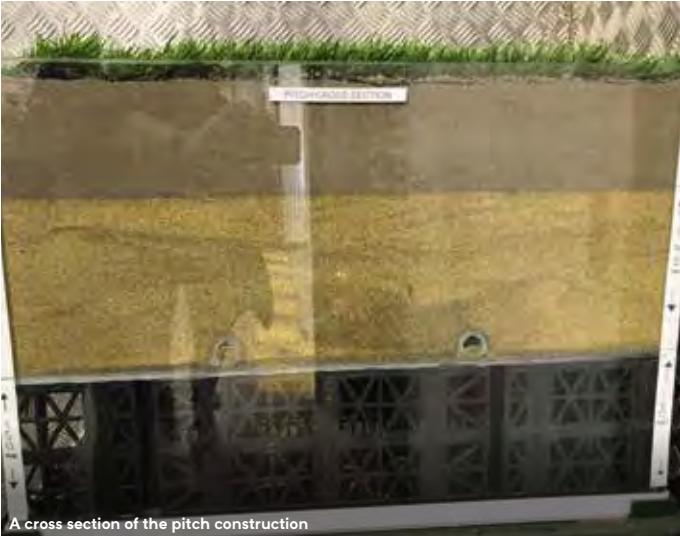
A cross section of the pitch construction
