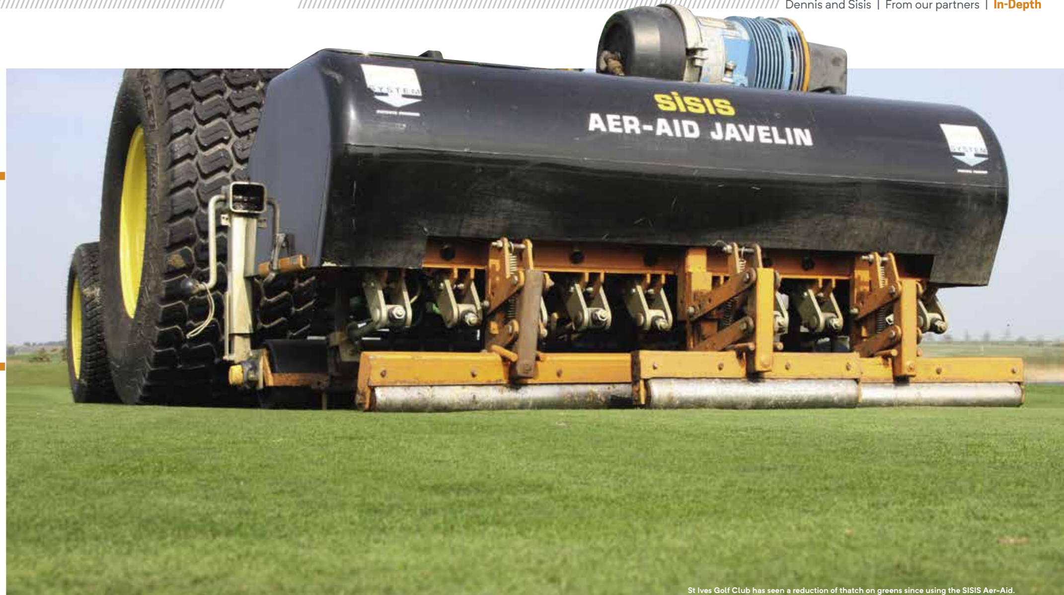
St Ives Golf Club has seen a reduction of thatch on greens since using the SISIS Aer-Aid.
