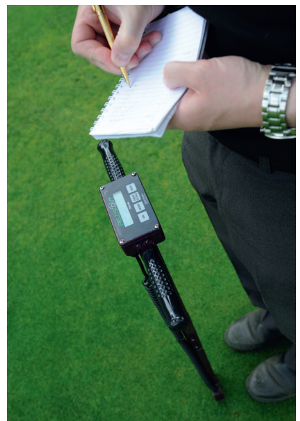
Moisture meter reading
