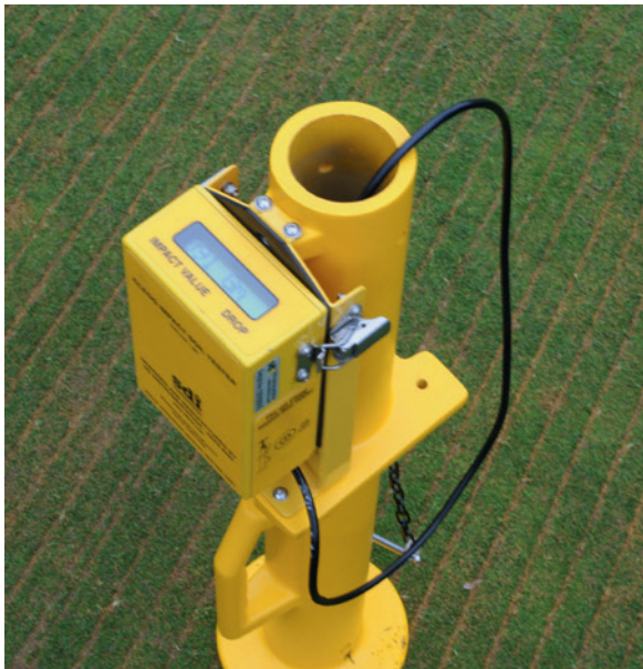
Clegg hammer measures firmness
