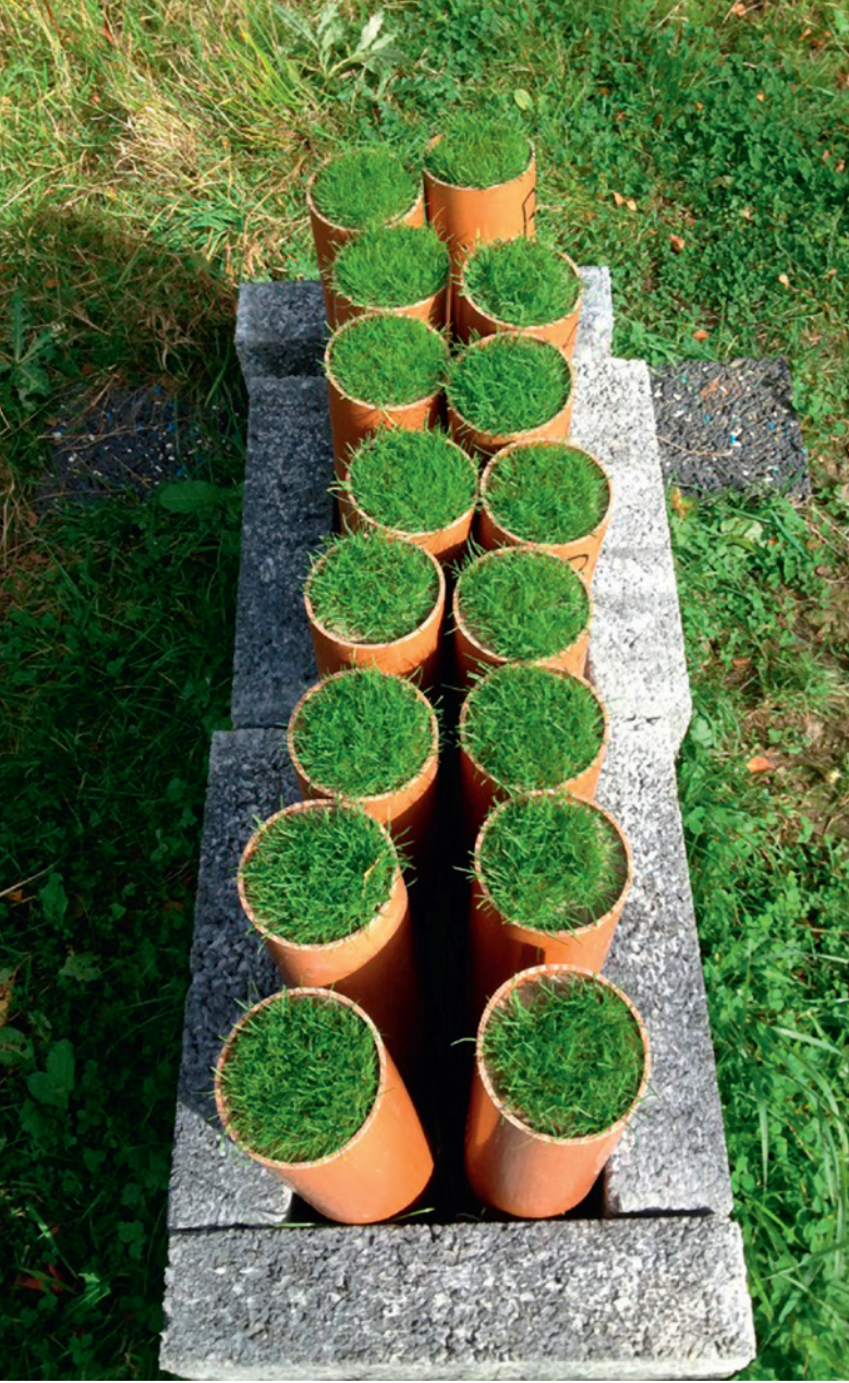
Growth tubes were designed to replicate USGA standards
