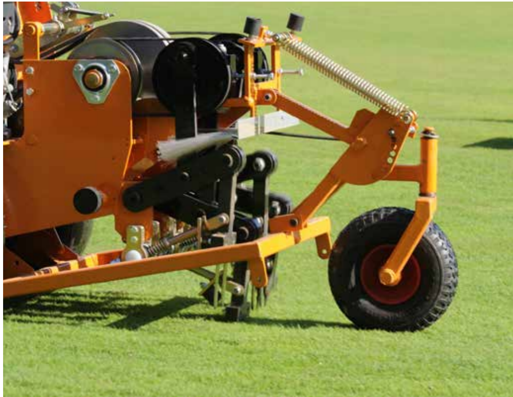
Above: The golf green is a pampered 'product' receiving dedicated nutrition and aeration provision (solid tine coring shown here) from the greenkeeper (Picture courtesy Syngenta)
