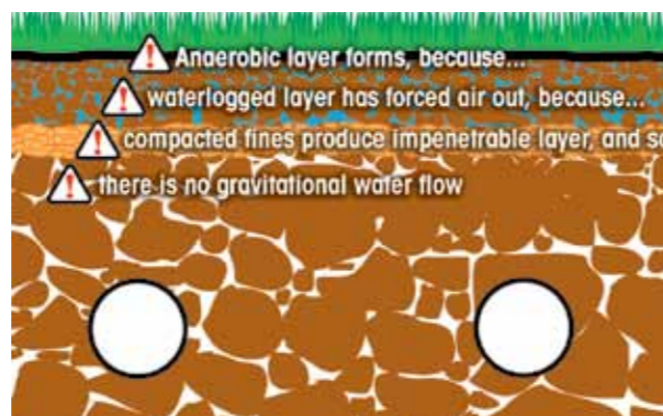
ABOVE TOP: Compaction clogs up pore spaces, preventing free drainage and air exchange. Anaerobic conditions force out oxygen and roots struggle to survive
