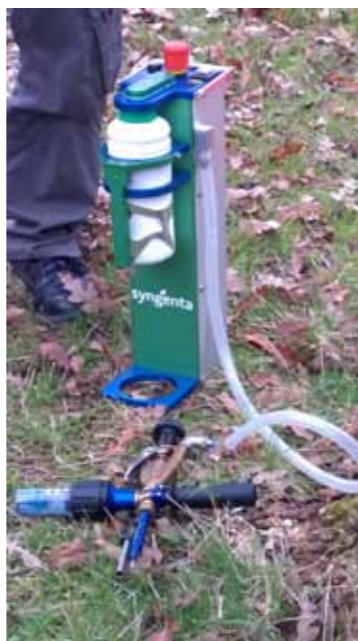
ABOVE: Syngenta Tree Micro Injection Kit used to experimentally treat an oak tree at The Richmond with systemically acting emamectin benzoate insecticide (Picture Courtesy Syngenta)
