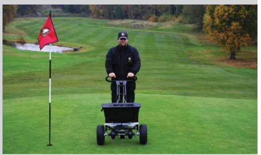
The Duo Spreader has a finely graded scale, allowing greenkeepers and groundsmen to control the exact dosage.
