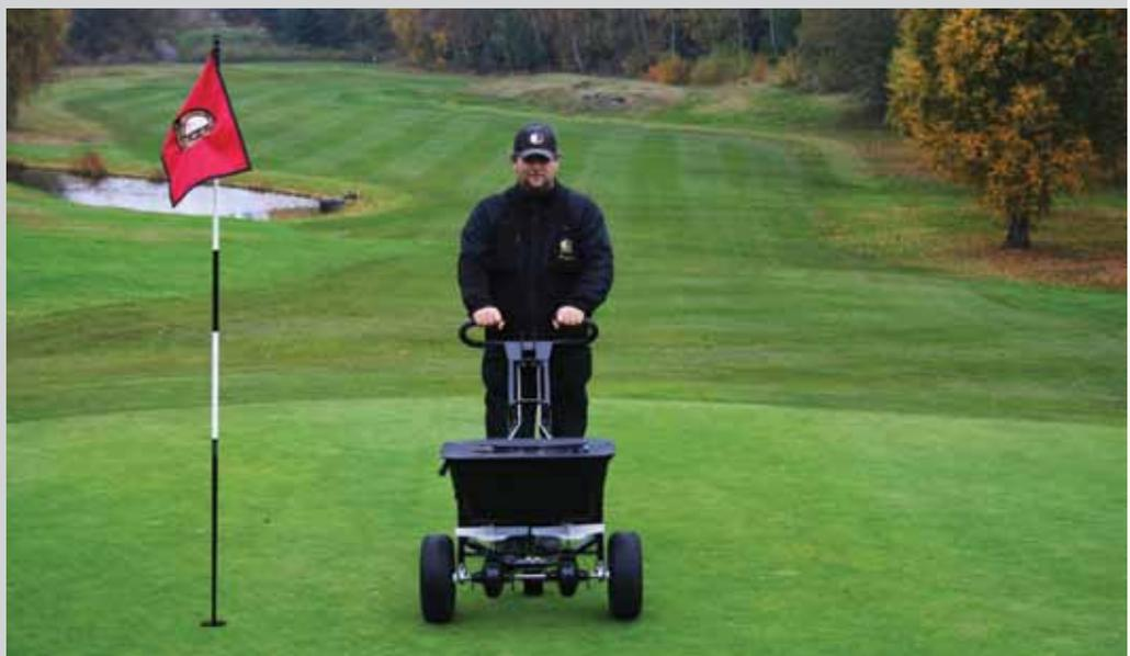
The Duo Spreader has a finely graded scale, allowing greenkeepers and groundsmen to control the exact dosage.
