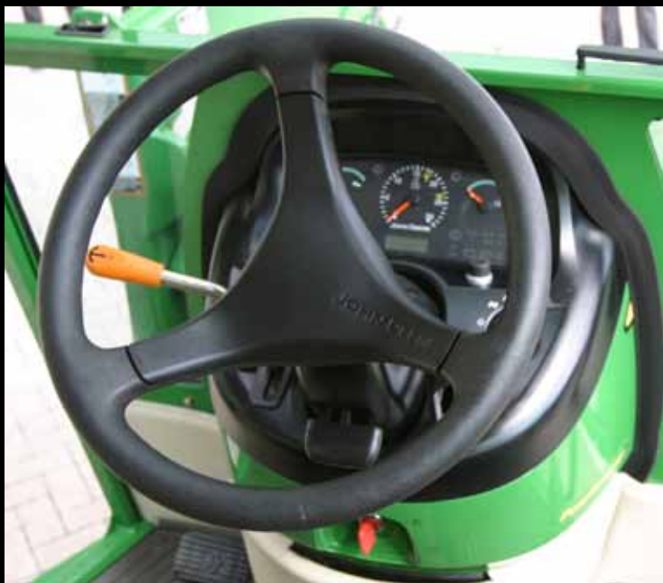
A shuttle forward and reverse lever makes changing direction much faster and is recommended for front loader work. The Power Reverser power shuttle on John Deere tractors allows the shift back and forth to be made without using the clutch.
