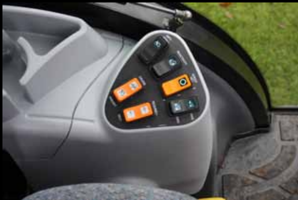
The New Holland EasyDrive CVT transmission is set up using a set of buttons mounted to the left of the operator. The main buttons are pretty easy to understand, with only Speed Set needing a bit of understanding. This control is essentially used to cap the tractors speed to 30%, 60% or 100% of maximum, in effect changing the sensitivity of the travel pedal to suit different applications.
