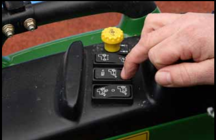
With the John Deere eHydro transmission, setting a fixed working speed is simple; use the travel pedals to attain the desired speed and press set. The speed can then be fine tuned, on the move, using the same switch.
