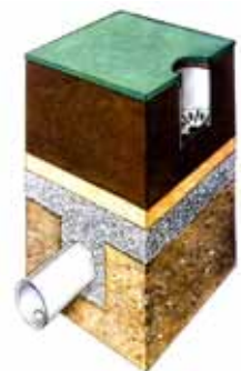
A soil modification procedure for greens involving a perched water table
