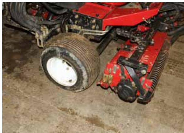
ABOVE: Ribbed tyres have replaced the original turf tyres on one of the Sidewinder mowers. This enables the unit to turn with minimal scuffing when mowing tees
