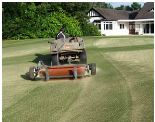
ABOVE: Brushing in top dressing using Greentek Multi-brush (Cotgrave Place) BELOW: Sweep n Fill brushing sand dressing into core holes (West Hill)
