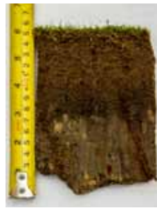
Low OM content and healthy ameliorated rootzone overlying the indigenous soil
