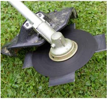
LEFT: A grass blade can tackle heavier growth than a line and, dependant upon design, also cope well with docks, light brush and bracken. There are so many designs of blade available that it is worth trying a few different types. The reversible four-blade unit pictured produces very little mulch and suits long grass that is raked and cleared separately.
