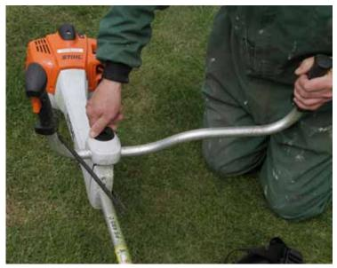
ABOVE: Modern cow or bike handle designs are 'offset' to the right, a degree of adjustment allowing the operator to set up the machine to suit personal preferences. Vibration control varies between makes and models, so it is worth trying a few alternatives; the best designs are much less tiring to operate over extended periods.
