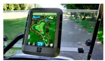
ensure that golf buggies are not driven off the property. Golfers are first alerted by a buzzer and on-screen messages, and the cart is automatically
