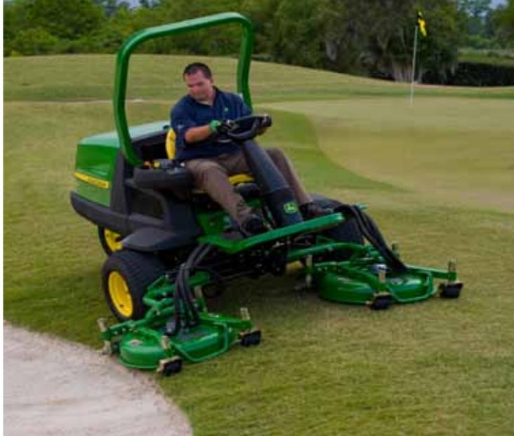
*John Deere 7400 mowers work at a variable width of 1.73m to 1.88m. The front units can be swung out when mowing next to a bunker to help prevent the mower's wheels damaging the edges. Each of the three units is 68.6cm in width*
