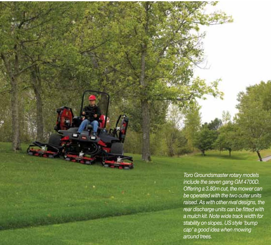
Toro Groundsmaster rotary models include the seven gang GM 4700D. Offering a 3.80m cut, the mower can be operated with the two outer units raised. As with other rival designs, the rear discharge units can be fitted with a mulch kit. Note wide track width for stability on slopes. US style 'bump cap' a good idea when mowing around trees.
