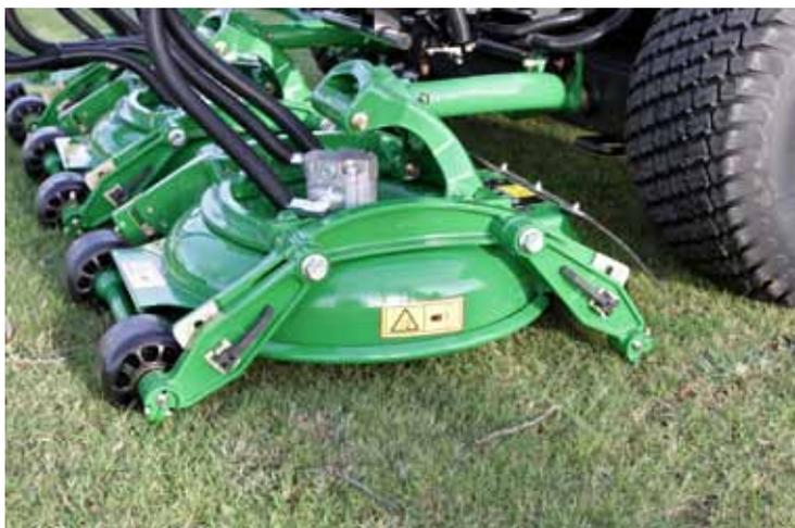
*Each measuring 53.3cm, the rear discharge cutting units fitted to the John Deere 8400 feature anti-scalp front- and full width rear-rolls to leave a striped finish. Designed to follow undulations, the units are 'narrower' than those of the JD 7400.*
