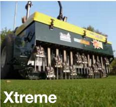
Shown at BTME for the first time were the Coremaster Xtreme aerators. These produce vertical aeration holes with no distortion or disturbance of any sports turf surface including fine turf or fairways.
