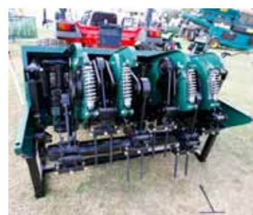
MAIN ABOVE: The Terrain Aeration Terralift injects air via 2.5cm probe and is claimed to send a blast of sufficient force to work down to around 1.0m. A Terralift can be used to inject dry materials to include dried milled seaweed, osmocote and slow release nutrients.
