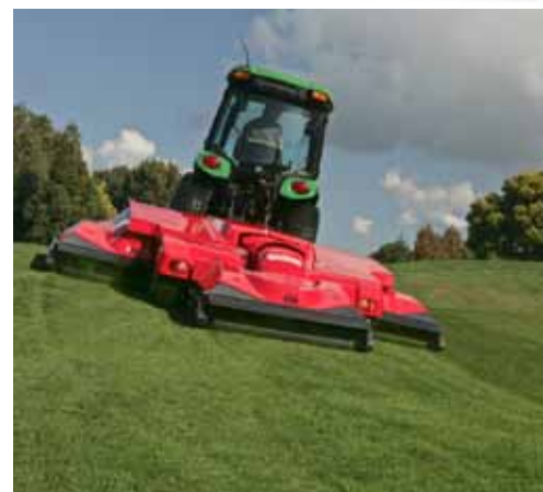
ABOVE: Traditional tractor trailed gangs still have a place on many golf courses, but for some a rotary alternative is preferred. The pictured Trimax Merlin is designed to produce a high quality finish over wide areas to include fairways.
