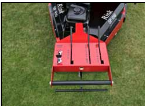
The Rink SP950 controls are simple, the operator engaging drive by raising the 'T' bar. In work, the units forward speed can be adjusted via the engine throttle, the unit proving simple to operate and match up between bouts passes.
