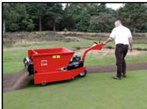
New to the UK, the pedestrian controlled Rink SP950 has a capacity of 0.33 m 3 and a spread width of 950mm. Powered by a 6.5hp Vanguard petrol engine, the units is ideally suited to spreading over small greens and areas of turf with restricted access.
