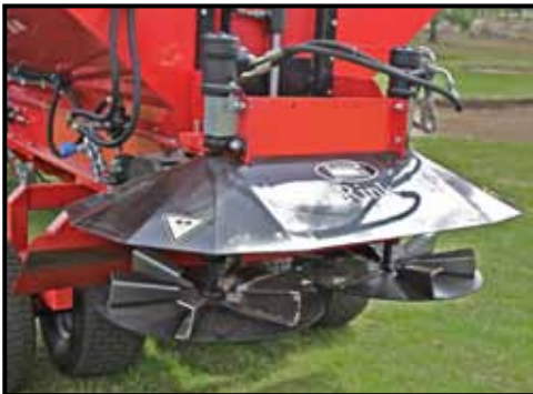
The contra rotating spinning discs can be set to spread at widths from around 2.0 to 12.0m, with variable application rates from light to heavy. Quick couplings enable the discs to be removed for direct dropping into a windrow for trench filling or be replaced with a cross conveyor.
