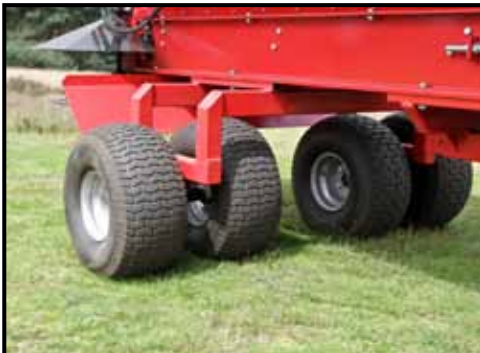
By spreading the load across four wheels, a trailed top dresser can offer a low ground bearing pressure. In the case of the Rink DS800, the four 24x13.00-12 tyres are inflated to 0.8bar.
