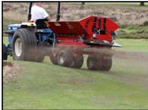
Swing axles ensure the wheels of trailed Rink DS models retain full ground contact over undulations. With any model of top dresser, the amount of material loaded can be cut down to reduce ground bearing pressures.
