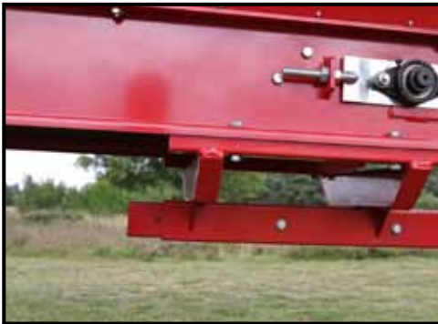
The drawbar of trailed Rink spreaders can be adjusted to suit the towing vehicle, the unit suiting tractors of 25hp plus with one double acting remote valve and delivering 25 l/min hydraulic flow.
