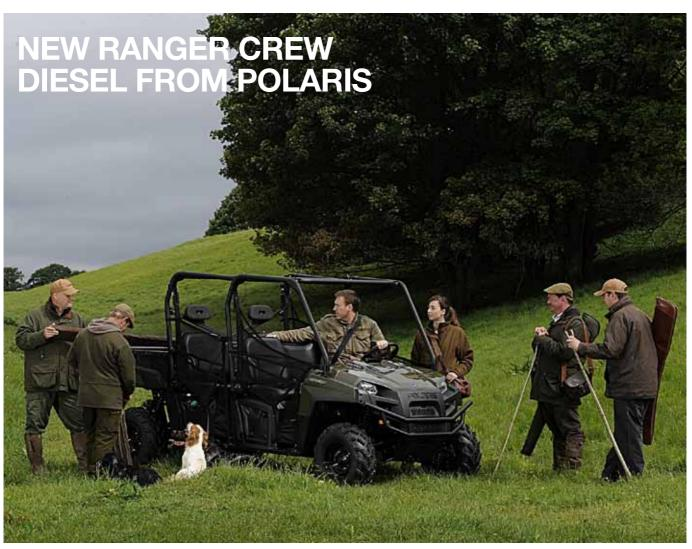
The new Polaris Ranger Crew diesel shares the 904cc, three-cylinder Yanmar diesel engine with the Ranger Diesel, coupled with the ability to carry six adults.
