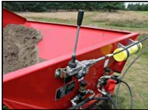
Pictured in its storage bracket, the single lever control for Rink DS top dressers will control the discharge conveyor; the rear discs continue to spin when the discharge conveyor stops. The conveyor, rear shut off and discs draw power from a single hydraulic outlet, this ensuring the unit cannot be operated without
