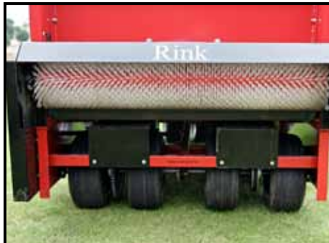
The Rink SP950 runs on six 13x6.50-6 tyres, four at the rear and two up front. The full width nylon brush helps ensure spread material is applied in an even layer and follows the same design as existing Rink top dressers.
