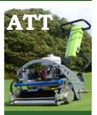
The Grass Group has unveiled the latest development from Advanced Turf Technology offering a progression for the INFiNiPower pedestrian drive unit which will now be available with an all new hybrid petrol/electric power unit. It incorporates a 1.5kw generator, coupled to a Honda GX-120 engine, to deliver a continuous 48V supply to both the traction drive and cutting cylinders' DC Brushless motors.
