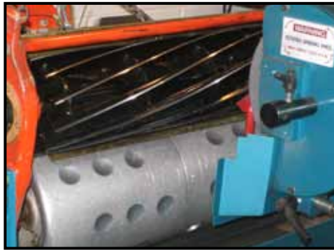
A grinder that allows a complete pedestrian mower to be worked upon will make the whole grinding task simpler.
