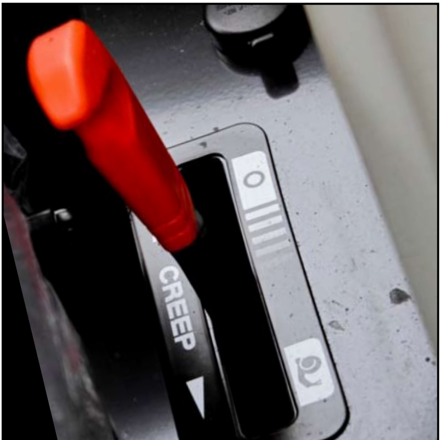
Creep speeds are selected via the separate lever above the main shift and provide a forward speed as low as 0.20km/hr. Once in the creep range, all eight speeds on offer are available
