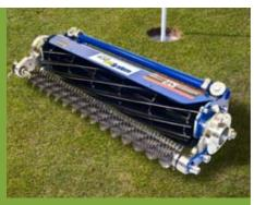
fairway mowers. This means that when cutting cassettes, they can be dropped out of the chassis and another set of TMSystem™ cassettes dropped in.
