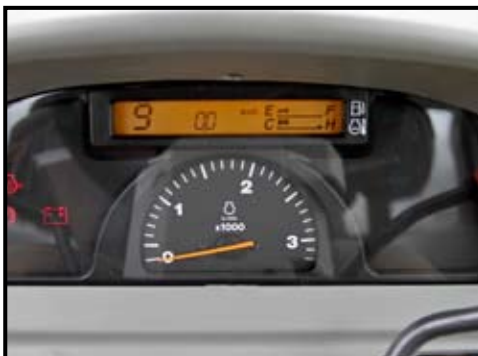
The IntelliPanel on GST L5040 tractors shows the selected gear on the left. In work, the gears can be swapped without using the 'clutch'. When the power shuttle is used to change direction, the clutch is again not required.
