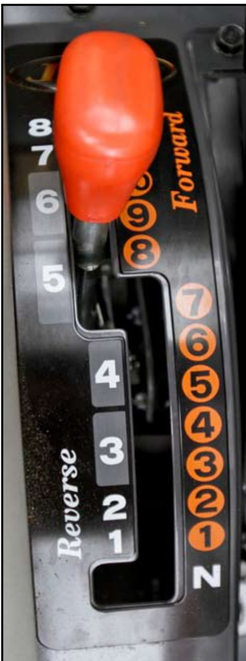
Swapping ratios on the GST transmission is simple; just move the gear selector to choose the desired ratio. This does not mean the tractor can be started in any gear but it does mean the operator can swap ratios on the move without using the clutch.
