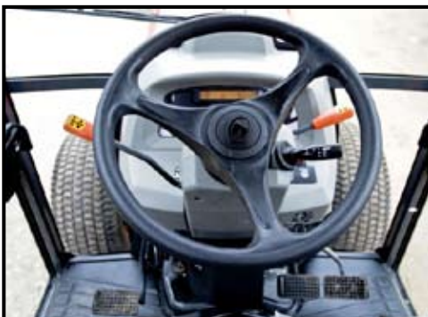
The dash of GST transmission models features a power shuttle lever to the left. The clutch pedal can be used when inching up to hitch attachments but otherwise can be pretty much left alone; drive engages as the engine is throttled up, with no need to use the clutch to swap ratios.
