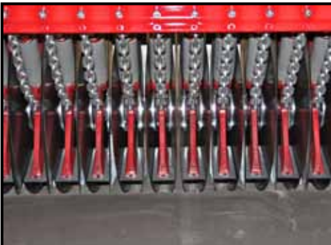
Metered seed is drip between the silt-cutting discs via tubes. Note inter-disc scrapers, the chain supports allowing the scraper to move out of the way and subsequently eject an object as the disc space opens up.
