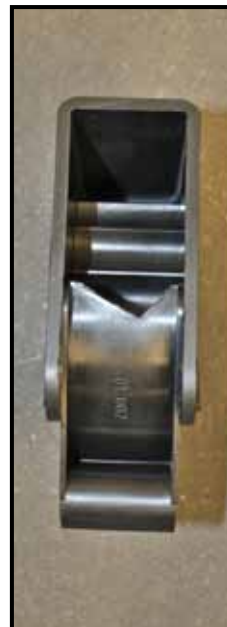
The flutes of the metering unit are partially covered by a flap, the aperture of which is adjusted to seed the seed and desired application rate.
