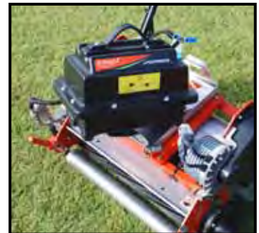
Battery powered pedestrian mowers are not new, but what has changed is the sophistication of modern units. A key emphasis is upon quality of cut, electronics enabling great precision when it comes to clip rate. Modern lead acid batteries also pack more power and staying power, reducing the risk of running out of puff half way through a job.
