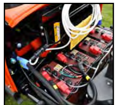
In full electric form, the Jacobsen Eclipse E322 is powered by six 8 volt batteries – two are mounted under the main pack of four - with a single point top up system making maintenance easier. A full charge should deliver 3 ¾ hours of running.
