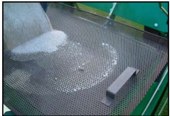
A simple screen is used to filter material entering the Graden sand hopper which requires a dry, free flowing in-fill material. This can include soil amendments such as Zeolite, porous ceramics (Profile etc) and Diatomaceous earth (Axis). Users suggest forcing clumps through the screen can cause blockages, the best approach being to allow anything that rests on the screen to either fall through on its own or be discarded.
