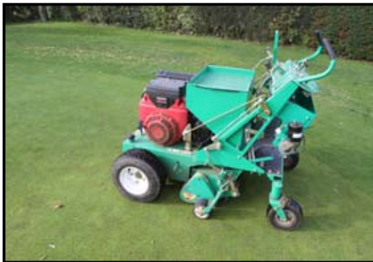
Powered by a 20hp Honda V-twin, the Graden Contour Sand Injection can be fitted with a Seeder Attachment. This allows seed to be sown while sand injecting. On a typical golf green, sole Graden Importers R and K Kensett suggest users are sowing bent seed at rates of 5g/m 2 when using the process in optimum conditions.
